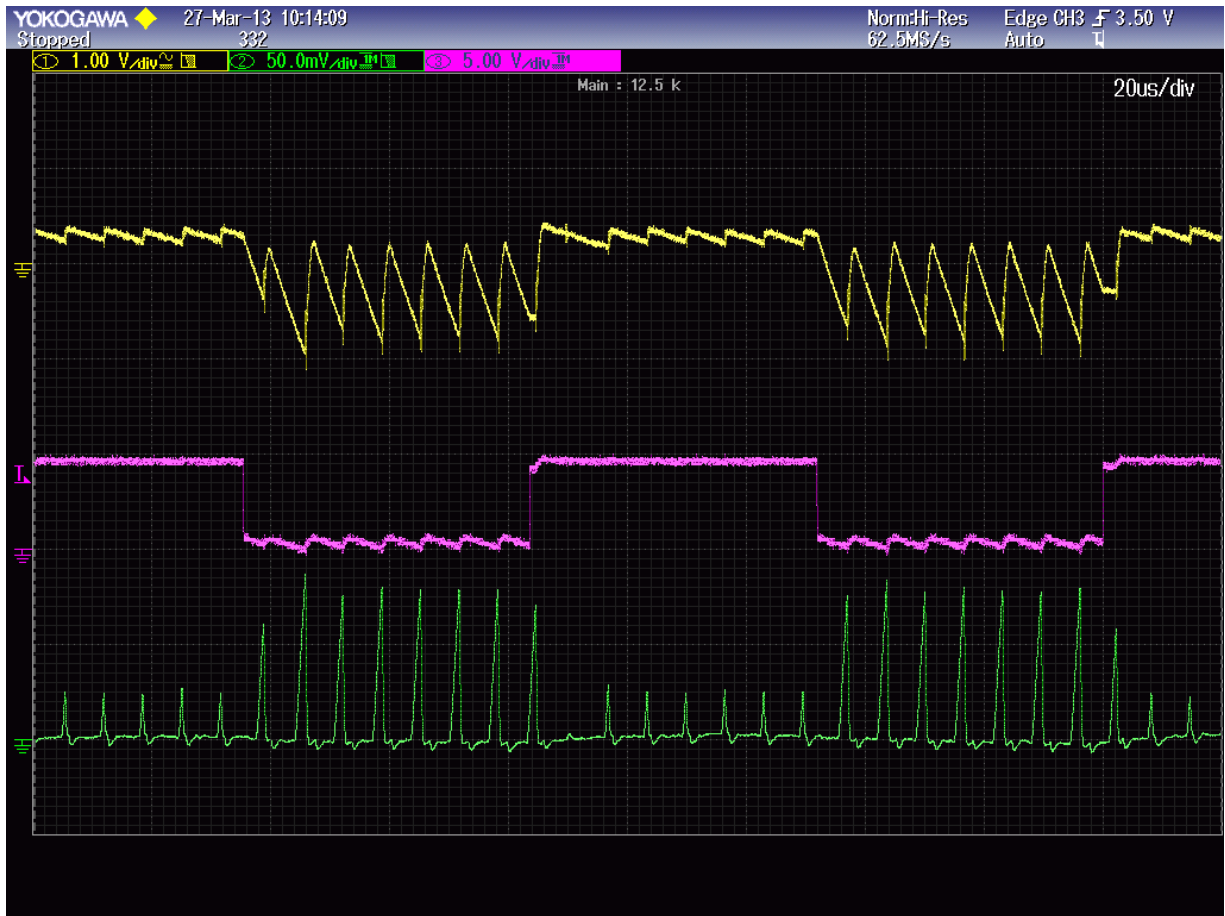
Figure 6 PEB Amplifier Running as a DC/DC Converter with a Step Load
