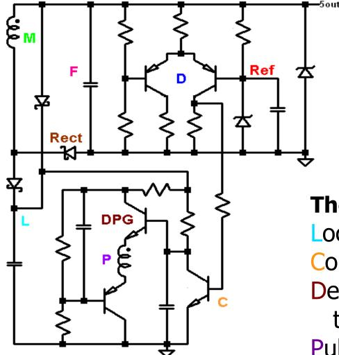
The upper block: Reference Differential error amp Main transformer secondary winding Rectifier and Filter
