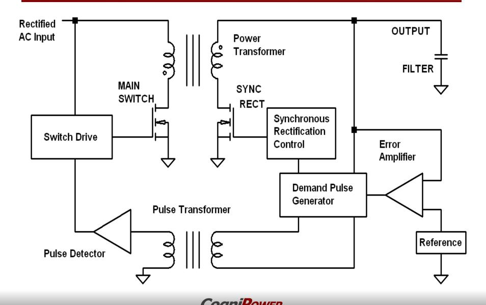
The primary-side switch is turned on by demand pulses sent through the pulse transformer
